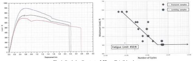
Fig-6: Static loading test – 3.75mm T.A.G implant.
