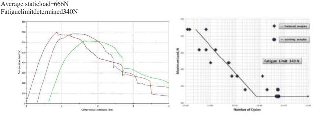
Fig-5: Static loading test – 3.3mm T.A.G implant.
