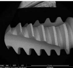
Fig-2: T.A.G implant thread shape
