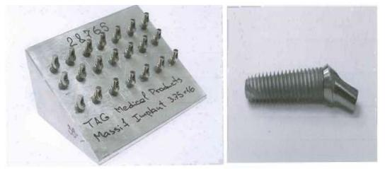
Fig-4: Testing bench for fatigue strength and tested implant.
