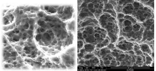
Fig-3: T.A.G implant micro surface (after modification)
